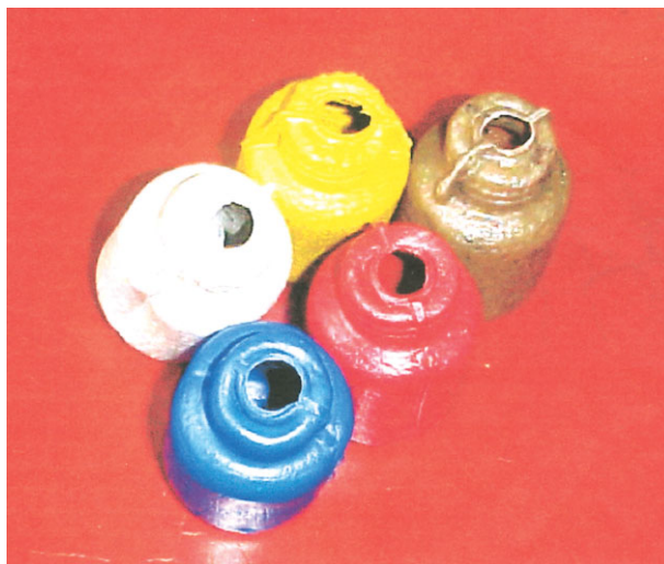
Figure 14 Picture of bottles made out of WPE/LDPE 70/30 blend through blow molding technique. [Color figure can be viewed in the online issue, which is available at www.interscience.wiley.com .]
